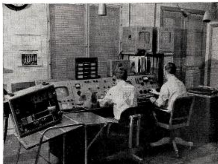
Two engineers control WNAO's entire program schedule—slides, film, studio and network—with Federal Transmitter Control Console and Poly-Efex Scanner providing complete transmitter supervisory control and audio/video switching. Scanner includes 2 slide sources, four-channel video switcher and "special effects" section.
